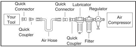
Figure 2. Typical filter/lubricator/regulator installation order.
